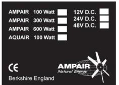
The label with the model type and nominal voltage is on the electrical box cover where the name Ampair is shortened to AMPAIR.
