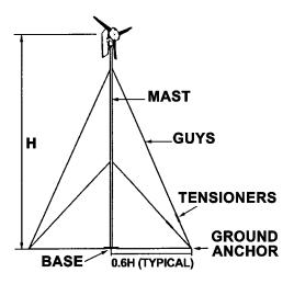
The top fixing point for the guys should allow for minimum overhang of the wind turbine generator, i.e. be only a
