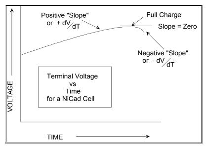
Enter the Benchmarq BQ2003 NiCad battery charger IC. This cell monitoring / charging IC performs all of the previously mentioned functions, and then some. This smart IC is the "doctor" in our NiCad recharging unit.
