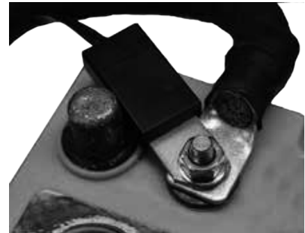
Fig 2.5(b) Temperature Sensor Installation
