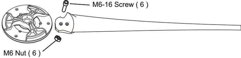
7). Remove the M16 nut from the rotor shaft. Slide the blades assembly onto the rotor shaft and place the nut on the shaft. DO NOT press the rotor shaft into the body.
