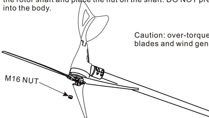
8). Insert the 8mm hex key into the rotor shaft and thread the nut on by spinning the blades assembly. Holding the blades assembly and tightening the M16 nut lightly with the 8mm hex key. Finally, spin the blades slowly to be sure they turn freely.
