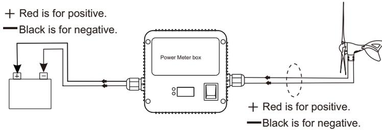
Use bolt driver to remove the 4pcs screws on the backside of the meter box and open it, then install the cables from the wind turbine and battery to the power meter box board as the following photo:
