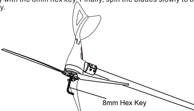
**CAUTION: DO NOT SCREW M16 NUT TOO TIGHTLY, OTHERWISE THE FACE BEARING WILL BE STUCK AND THE BLADES ROTATE DIFFICULTLY!**
