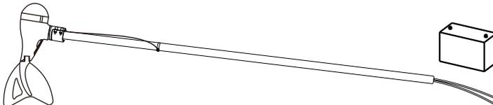
6). Place one of the blades on the hub socket and insert one of the M6-15 socket head cap screws. Place a plastic disk on the end of the screw, then place self-locking nut (M6) and tighten it with the 5mm hex key to 8-10 foot lbs. (10.5-13.5 N.m). Repeat this procedure on all three blades.
