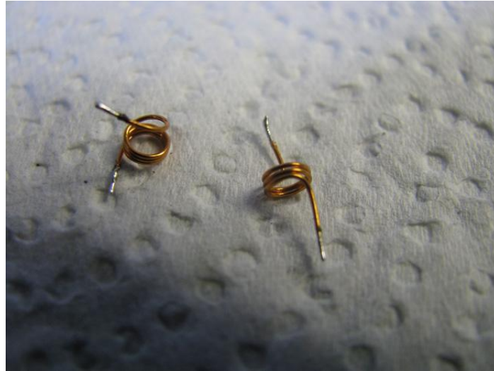
Fig 15 the 23cm inductors L1 and L2
