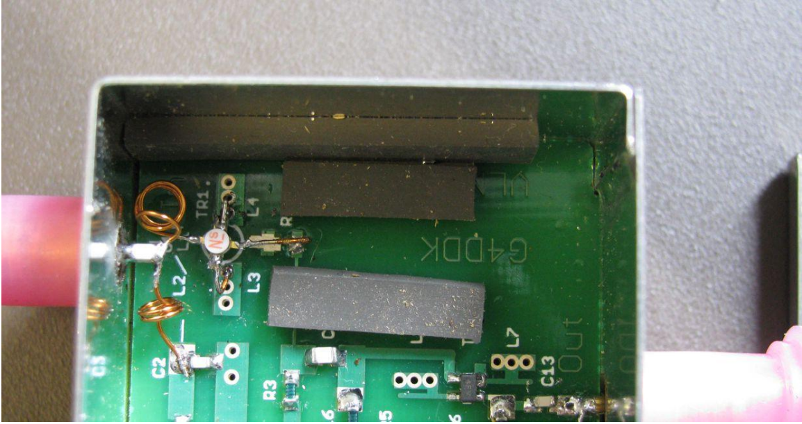
Fig 17(a) 23cm input inductors and placing of the absorber
