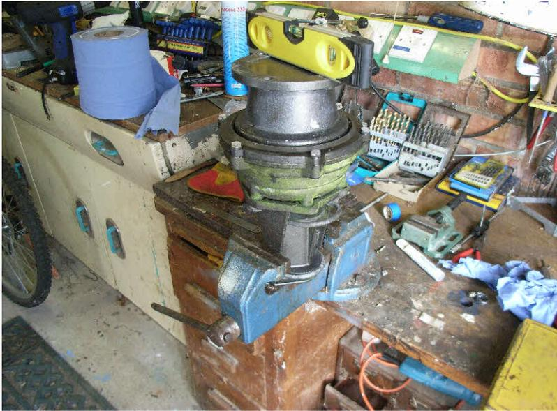
The rotator is mounted in a vice bell down, and the motor housing is marked to show it's position in line with the bell housing. All settings must be maintained and the gear train not rotated if the direction indicator potentiometer is not to be disturbed. Keep it level!
