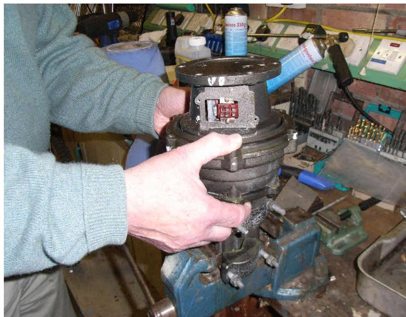
Holding the now un-bolted lower ball race with both hands invert it and place it in a tray standing on the bottom flange of the motor housing. Gently drop the ball race holder to the tray with the balls still loaded. If your rotator is like mine, the grease will need to be cleaned off and the ball race re-greased.
