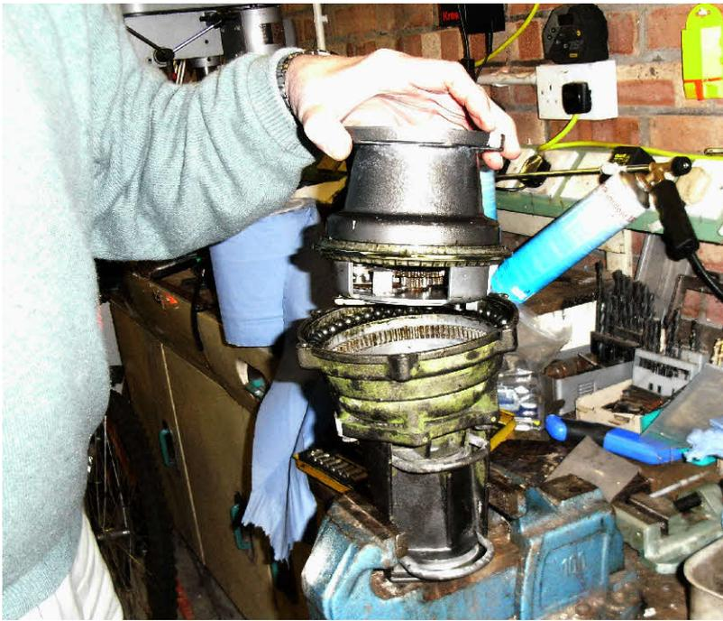
With both hands holding the motor housing in place, invert the rotator so the bell housing is at the bottom and refit in the vice. Note, the motor housing must be refitted in the same line as the bell so make sure the markers are clear. Lift the motor housing to reveal the second ball race. Some balls may be held by the grease to the motor housing so ensure you do not lose any.
