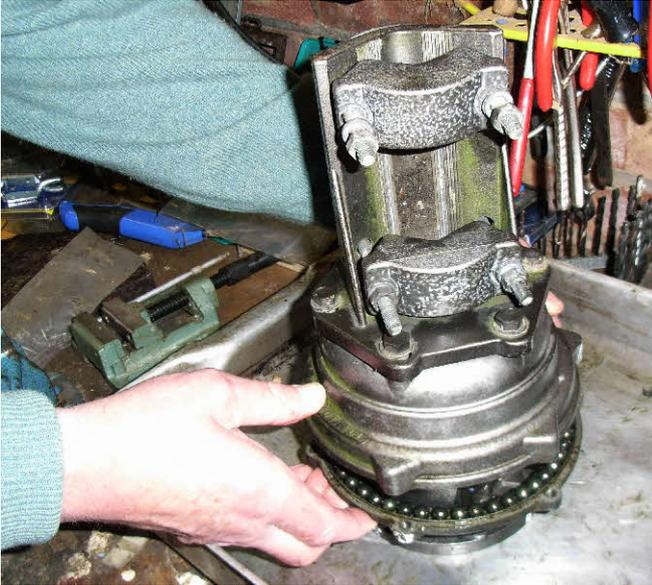
Showing the ball race holder being lowered on to the tray.
