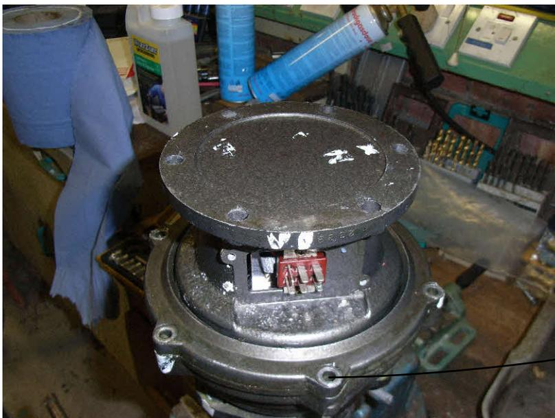
Remove the 6 bolts holding the lower ball race holder. Do not lift off yet it or the balls will drop out!
