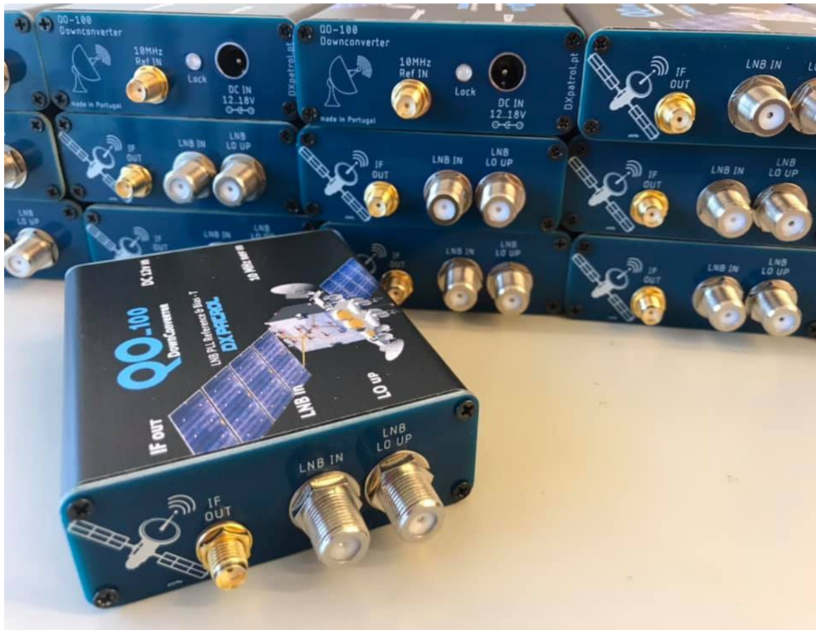
Fig 1 a complete boxed Down converter
