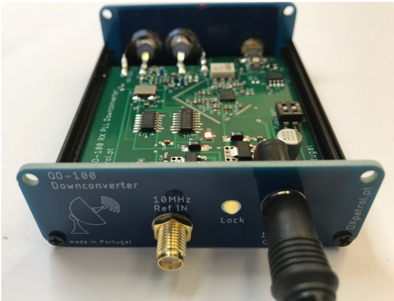
Fig 7 Orange LED = PLL LOCKED
