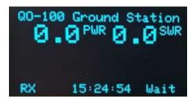
RX mode, no Power/SWR detected, Clock and Wait.
