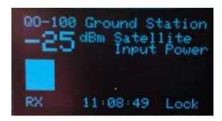
This page shows input satellite strength. This is shown in dBm and it's very useful to point the dish and fine adjustment of LNB in the focal point.
