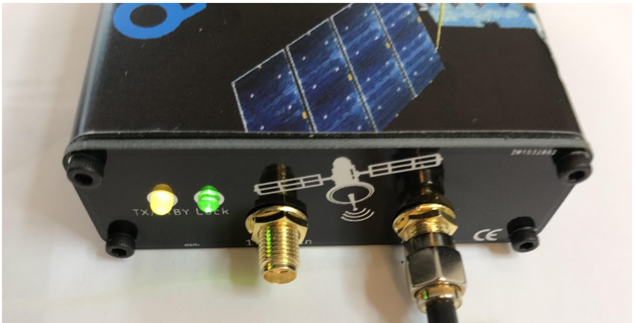
Fig 4 TX mode, TX/STBY led is Orange
