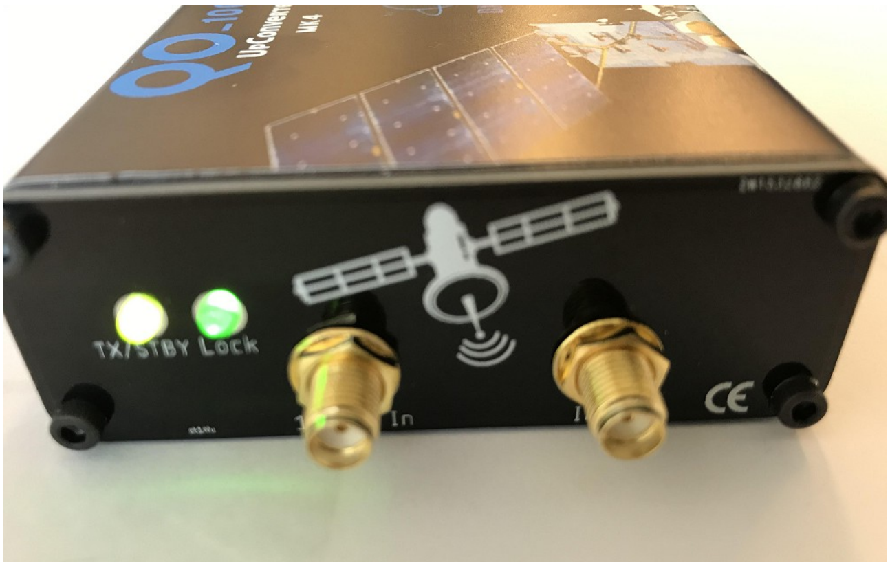
Fig3 Standby mode, Lock Led Green and TX/STBY Led Green.
