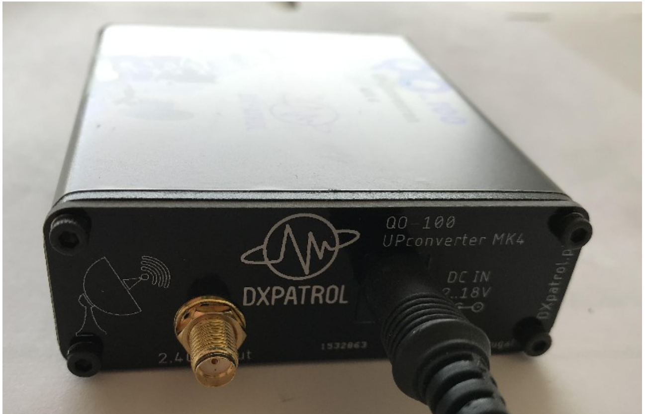
Fig 2 DC connection, (positive to center pin)
