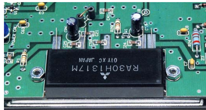
Figure 36. RF PCB attached to the RF Power Module Screws.
