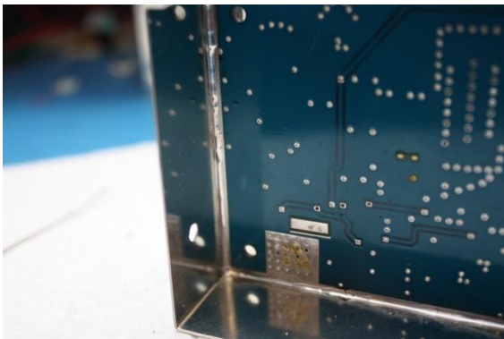
8a PCB offered up to first side of box (IF end) and tack soldered in 2 or 3 places along the 22mm line on both end wall and side wall.
