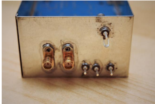
Photo 10. IF Connectors and feed-throughs soldered to the box end wall
