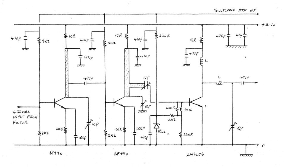
MMT 432/144 OSCILLATOR AND MULTIPLIER STAGES
