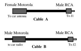
*Cable A:* Cable A is used to extend the existing automotive antenna lead to reach the converter enclosure. One end is a Motorola female connector to mate with the male connector on the antenna cable. The other end of the cable is terminated with a solder-on RCA male connector to mate with jack J1 (antenna) on the VEC-101K. The cable can be made by cutting the male connector off of
