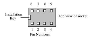
□ □ 2. Install and solder the 8-pin IC socket at location U1. Observe proper orientation!
