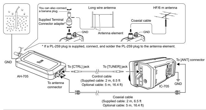
NOTE: The antenna tuner must have an adequate ground connection. Otherwise, the overall efficiency of the transceiver and antenna tuner installation will be reduced. Interference, RF feedback, and electrical shocks from other equipment could also
