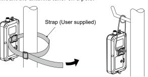
You can hang the antenna tuner, by threading a piece of cord through the bracket.
