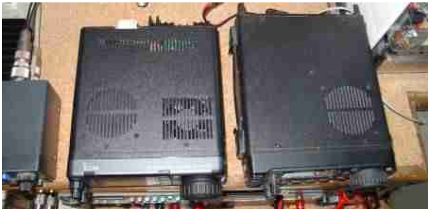
The IC-7000 on the left (notice the fan) and the longer IC-703 on the right!
