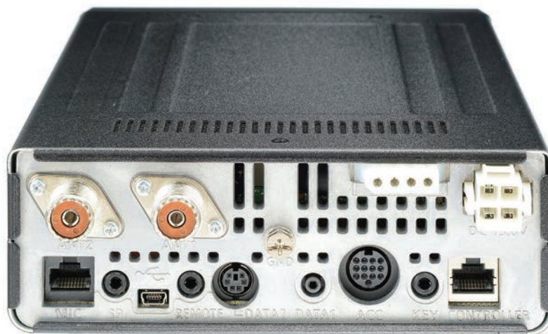
Figure 1 — The Icom IC-7100 main unit rear panel will look familiar to owners of recent Icom transceivers. It has connections for interfacing with a computer, external power amplifier, antenna and station accessories, as well as mic and speaker jacks and an Ethernet-type connector for the control head cable.
