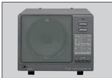
SP-20 EXTERNAL SPEAKER 4 audio filters; headphone jack; can connect to 2 transceivers. Input impedance: 8Ω Max. input power: 5W
