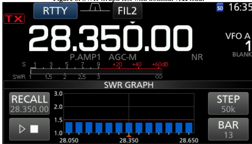
Figure 8: SWR Graph test with nominal 75Ω load.
