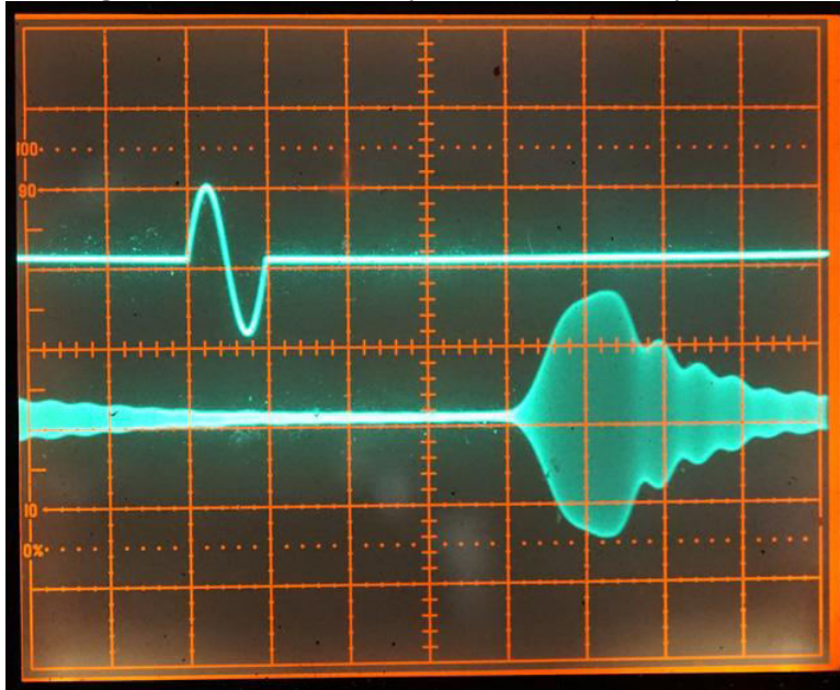
Figure 36: Transmit latency, MID TBW. Latency 4.2 ms.
