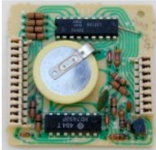
It is a well known fact that the RAM boards in some of the older ICOM radios have in them have volatile memory contents which need a lithium battery backup. The data in this RAM retains as long as the battery works fine. Usual life of this factory installed battery is between 7 to 15 years, depending on the working and storage conditions of the radio. There is no evident problem if the battery is replaced in time. You could replace the battery by using the procedure mentioned in this Icom URL :
