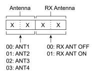
① If the Antenna Type is set to "RX-I/O," command "01 (RX ANT ON)" is invalid and "00 (RX ANT OFF)" is always returned.
