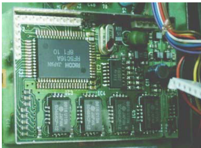
The opened CRTC module; C11 is the blue cap, to the right of the CRTC module.
