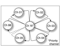
watch pauses until the signal disappears; when a signal is detected on a channel other than the Priority channel, the Priority watch switches to Dualwatch, until the signal disappears.
