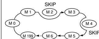
Repeatedly scans memory channels except those set as skip channels. Skip channels can be turned ON and OFF by pushing **[FUNC] + [V/M]** (**SKIP•S.MW**) in *memory mode*.
