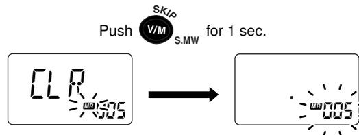
While pushing and holding **[FUNC]**, push and hold **[V/M] (SKIP•S.MW)** for 1 sec. after step ② also clears the memory contents. In this case, steps ③ and ④ are not necessary.
