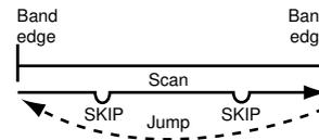
Skips unwanted frequencies or channels that inconveniently stop scanning. This function can be turned ON and OFF by pushing **[FUNC] + [V/M]** (**SKIP•S.MW**) in either VFO or *memory mode*.
