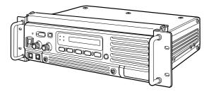
⑧ Turn the repeater upside down, then removing the 4 legs for mounting the 19 inch rack.
