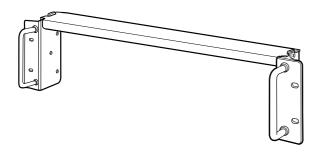
(5) Remove the 2 screws (M4  $\times$  8) from both side of the side panel (front-end).
