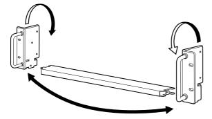
③ Attach the handles to the bar, then tighten the screws.
