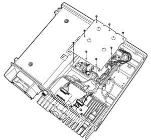
③ Replace the circuitry fuse as shown below.
