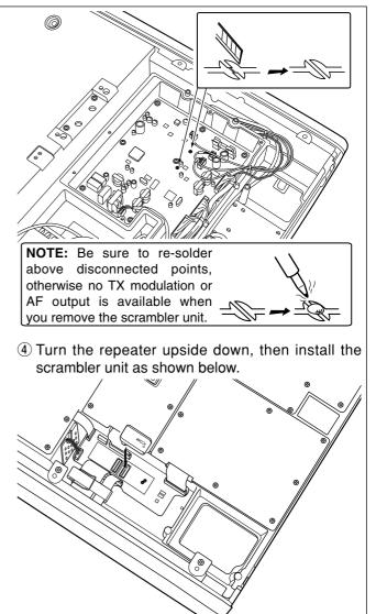
(5) Return the LOGIC shielding plate, top and bottom covers to their original positions.
