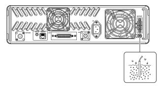
$\triangle$  **WARNING: NEVER** connect the [GND] terminal to a gas or electric pipe, since the connection could cause an explosion or electric shock.
