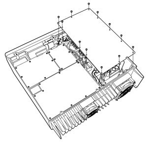
3 Replace the circuitry fuse as shown below.
