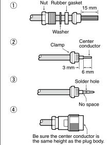
Slide the nut, flat washer, rubber gasket and clamp over the coaxial cable, then cut the end of the cable evenly.
