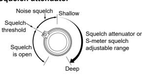
The transceiver has an RF attenuator related to the squelch level setting. Approximately 20 dB of attenuation is obtained at the maximum setting.
