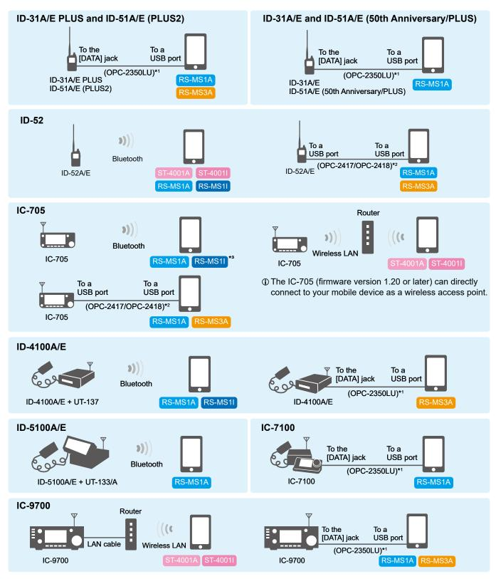
\*1 The OPC-2350LU that connects to the DATA jack of the transceiver is supplied the two types of USB cable, for an Android device (USB mini-B/USB micro-B) and a PC (USB mini-B/USB Type-A).
