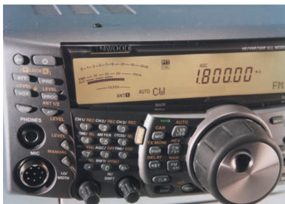
● Fig. 1: Close up view of the very clear, simple and straightforward l.c.d. main display, showing the multi-function meter. The selected DSP filter parameters are displayed under the Filter logo in the form of bargraph segments (see text).
