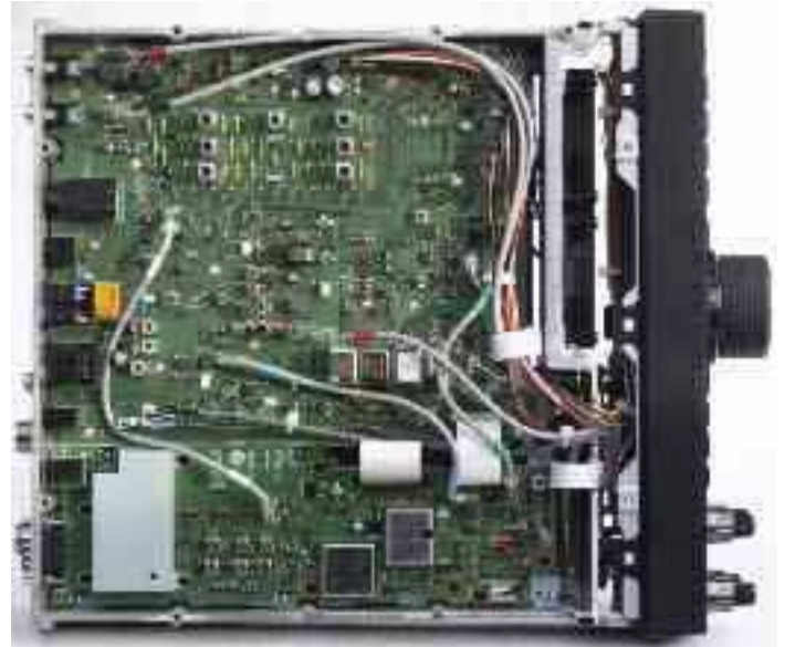
PHOTO 3: Underneath view showing signal processing boards.
