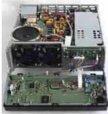
PHOTO 5: The front panel hinged down showing the PA cooling fans.
