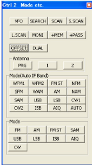
CONTROL 2 (receive mode, etc)
