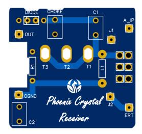
$1 \times PCB$  (this is the main part of the radio kit) L1 Antenna Coil (See Instructions) 1N34 Point Contact Diode (or equivalent) Choke 10mH C1 10pF Disk C2 1nF (Green) Antenna type Switch R1 33K or 36K  $\frac{1}{4}$  watt Resistor 4 x Sockets 1 x Front Panel 1 x Case 1 x Tuning Knob Foam Tape Mounting screw set Headphone Socket Socket wires
