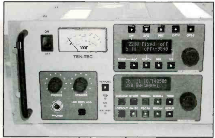
The left side of the receiver features the memory and operating sections, as well as the signal strength meter. Note the dual volume controls for speaker and headphones.
