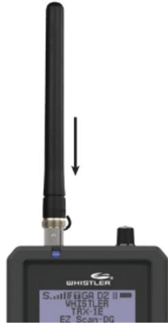
You can use a variety of antennas. To connect an external antenna, follow the installation instructions supplied with the antenna. Always use 50-ohm coaxial cable, such as RG-58 or RG-213 low-loss dielectric coaxial cable. You may also need a BNC adapter.
