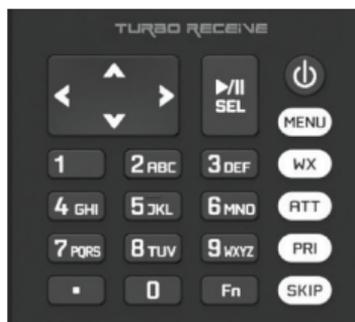
**POWER** - press and hold
