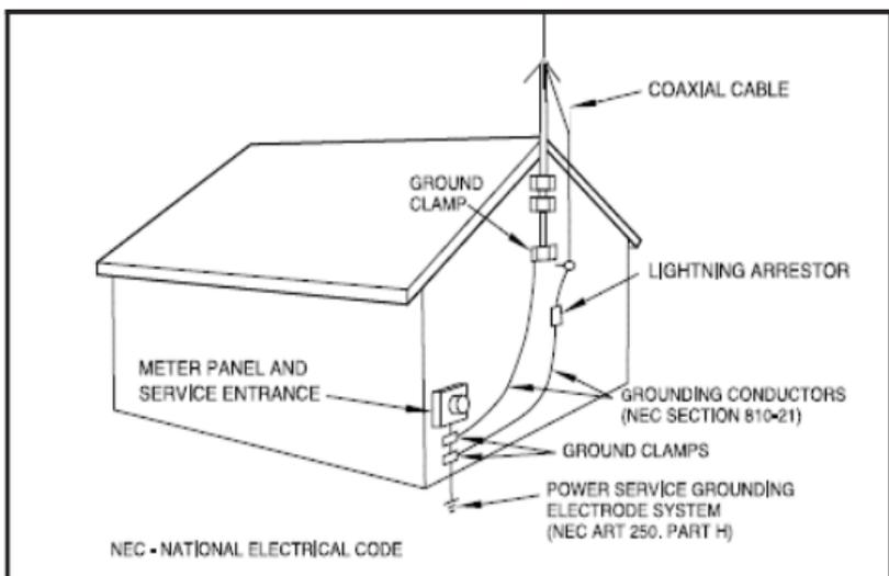
**WARNING:** Outdoor antennas must be properly grounded to prevent static buildup and lightning damage. Article 810 of the National Electrical Code, ANSI/NFPA 70, provides information about proper grounding of the antenna mast, connection of coaxial cable to a lightning arrestor, size of grounding conductors, location of the lightning arrestor and connection of grounding conductors to grounding electrodes.
