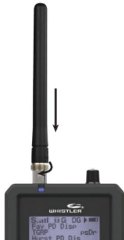
You can use a variety of antennas. To connect and external antenna, follow the installation instructions supplied with the antenna. Always use 50-ohm coaxial cable, such as RG-58 or RG-8 low-loss dielectric coaxial cable. You may also need a BNC adapter.
