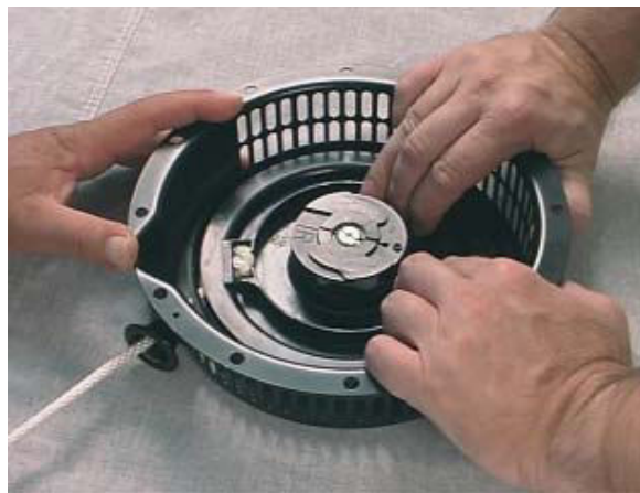
Figure 4-3. Recoil Starter Replacement – Aligning Rope Access
