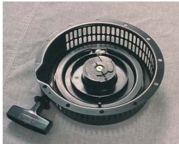
Figure 4-6. Recoil Starter Replacement – Recoil Replacement Rope
