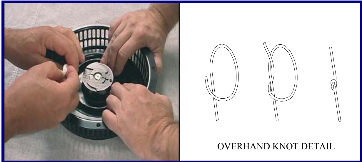
Figure 4-5. Recoil Starter Replacement – Knotting Rope
