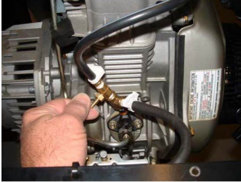
Figure 2-1. Initial Starting Procedure – Opening Bleed Valve
