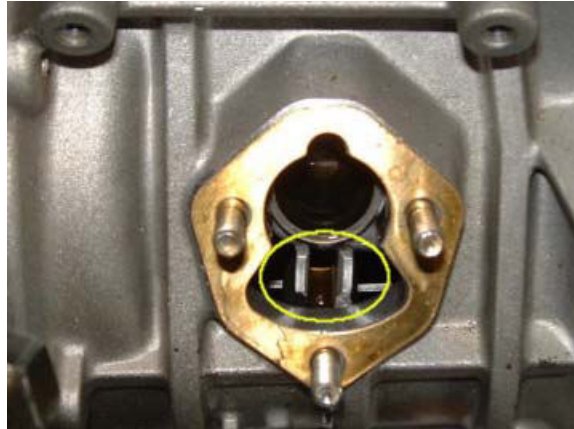
Figure 4-14. Free Injector Pump Piston – Shutoff Valve, Correct Placement
