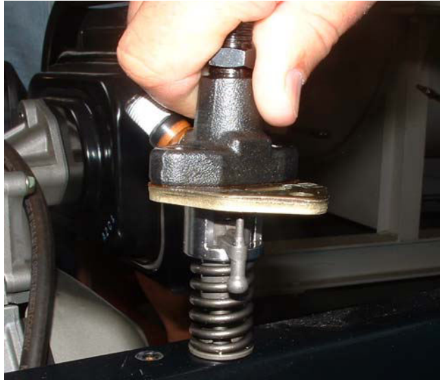
Figure 4-13. Free Injector Pump Piston – Free Piston
