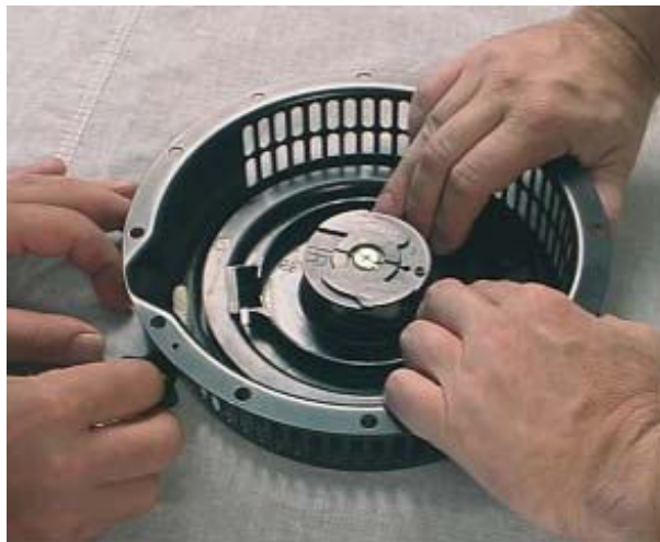
Figure 4-4. Recoil Starter Replacement – Feeding Replacement Rope
