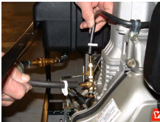
Figure 4-8. Free Injector Pump Piston – Removing Fuel Supply Line
