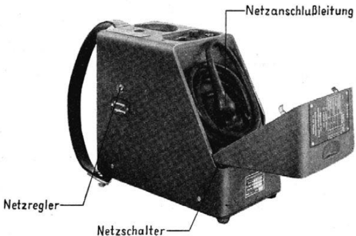
Figure 4 Tube Tester with mains lead coiled inside
