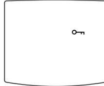
**Reference:** When the keys are locked, only the PTT and the MONI keys are active. All other keys are inoperative. Transmitting and monitoring operations are possible even when the key lock function is activated.
