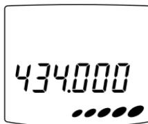
The S meter indicates the unit is in the transmitting mode.
