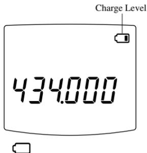
When the charge level becomes low, an empty battery mark appears. Charge (or replace) the battery.
