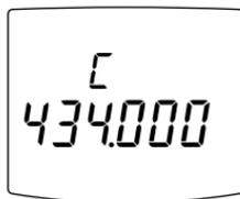
2. Press the V/M key to return to the VFO mode or the Memory mode.
