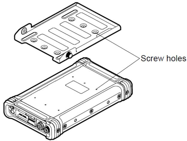
3. Secure the bracket with six M3\*6 screws.
