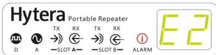
When this alarm segment is displayed, the repeater will still work properly and will power off automatically when running out of power.
