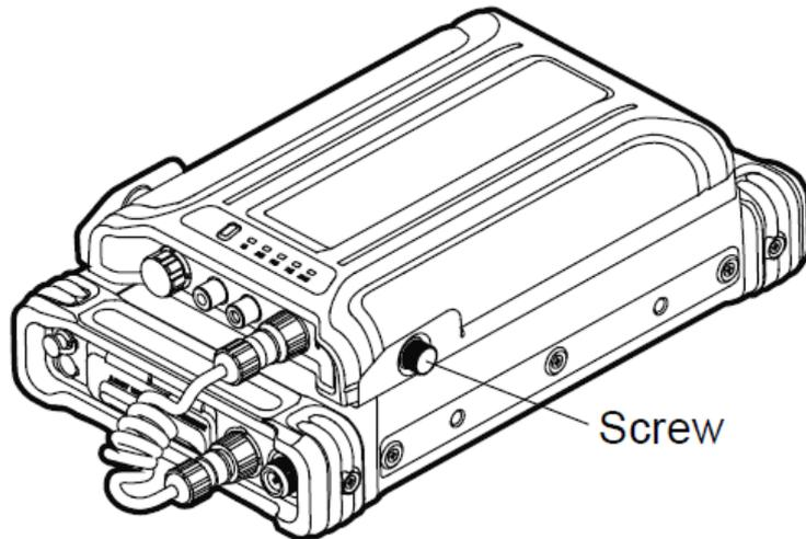
1. Plug the aviation plug (female) of the power cord into the power input of the repeater and fasten the screws on the plug.
