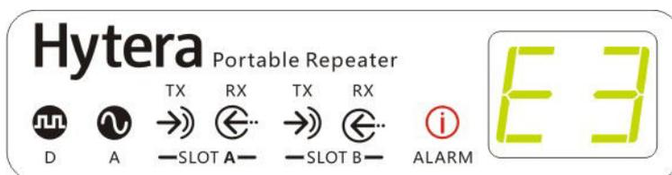
When this alarm is given, the repeater cannot work properly and will power off automatically in 3s. If the repeater returns to normal operation within the 3s, the alarm will be eliminated so that the repeater will not power off.
