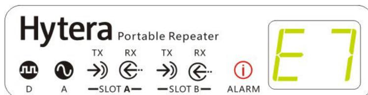
When this alarm is given, the repeater can still work properly.
