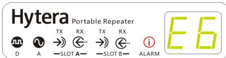
When this alarm is given, the repeater can still work properly. During a rise in ambient temperature, the repeater will keep track of the Tx power with adjustments in order to lower the temperature.
