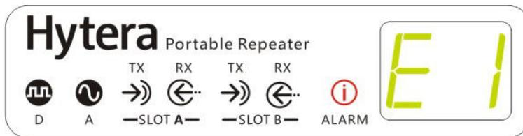
When this alarm is given, the repeater cannot work properly and will power off automatically in 3s. Then please ask your local dealer to replace the power supply management system or for further help. If you switch to an external power supply, this alarm will be eliminated with the segment disappearing and the alarm indicator going out.
