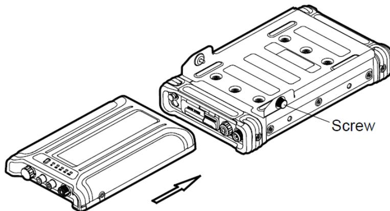
2. Fasten the screws on the bracket to secure the system.
