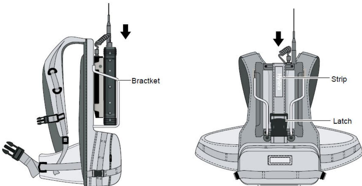
**Step 4** Hang the remote speaker microphone (SM18A1) on the strap of the backpack (optional) as shown in the following figure.
