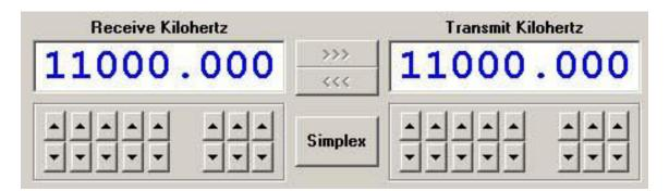
**Simplex** button allows selection of **Simplex** (Same TX and RX frequency) or **Duplex** mode. (Difference TX and RX frequency)
