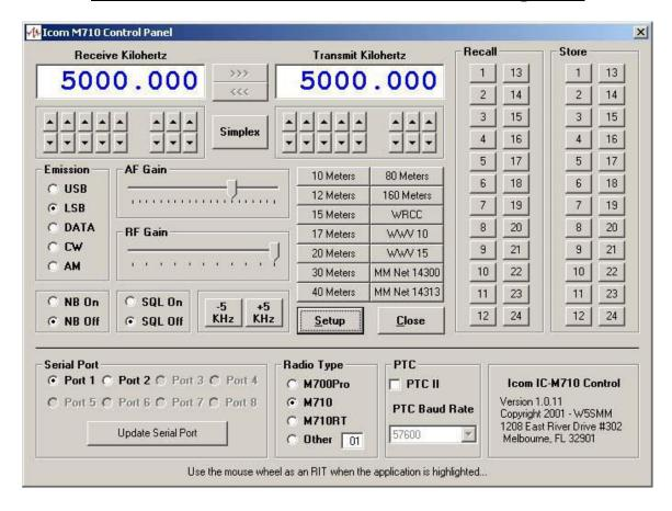
M710 control program is an easy to use program that makes using your ICOM HF-SSB Marine radio as convenient as using a Ham radio. Its supports the ICOM M700Pro, M710 and M710RT HF, SSB Marine radios.
