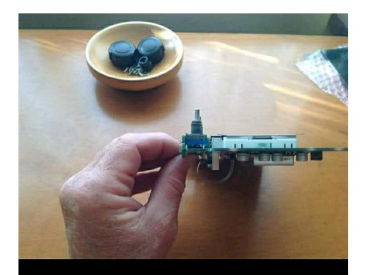
As you reassemble, make sure the knob pots are straight so they locate back through the main housing, do not force anything!
