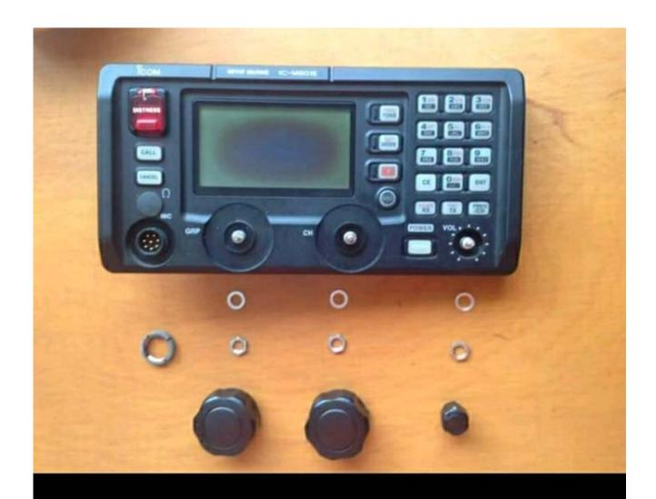
First I removed the knobs, nuts and washers.
