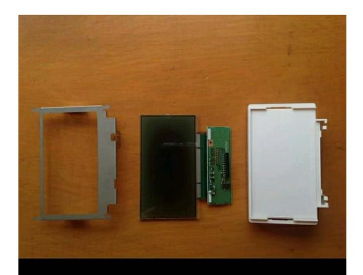
All apart, reassembly is exactly the opposite of removal. Note there is a white card that sits behind the screen, located in the white housing. Make sure the screen and inner face of the housing are spotless before you reassemble, it would bug you for ever if there was a bit of fluff in there.
