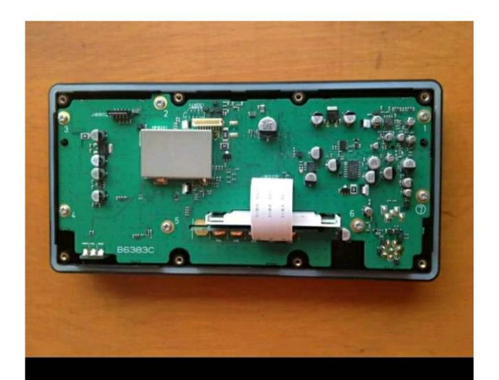
Remove the seven screws, numbered, and lift off the main board carefully.
