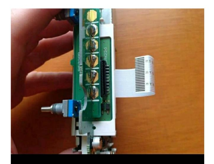
Do this very carefully, I used a pencil inside the ribbon with two thumbs on the ribbon to ease it off.
