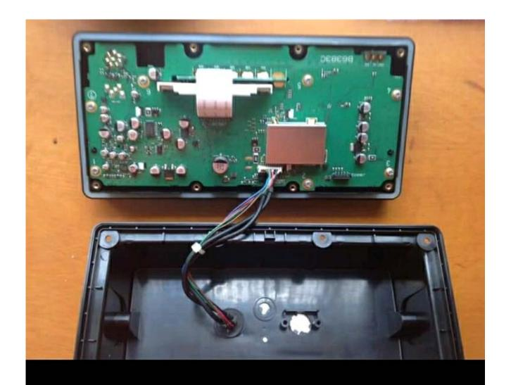
Remove the eight screws holding the back on and unplug the wiring harness from the board.
