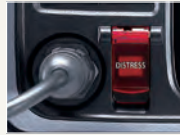
Distress button with a spring-loaded cover
