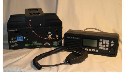
The SEA 245D system consists of one 2451D RTU and up to four 2450 Remote Control Heads. Its flexible design and reliability provide optimal capabilities for all radiotelephone Operators. The SEA 2451D is a highly integrated and compact solid state MF/HF SSB transceiver housed in a ruggedized chassis specifically designed for long duration transmit cycles.
