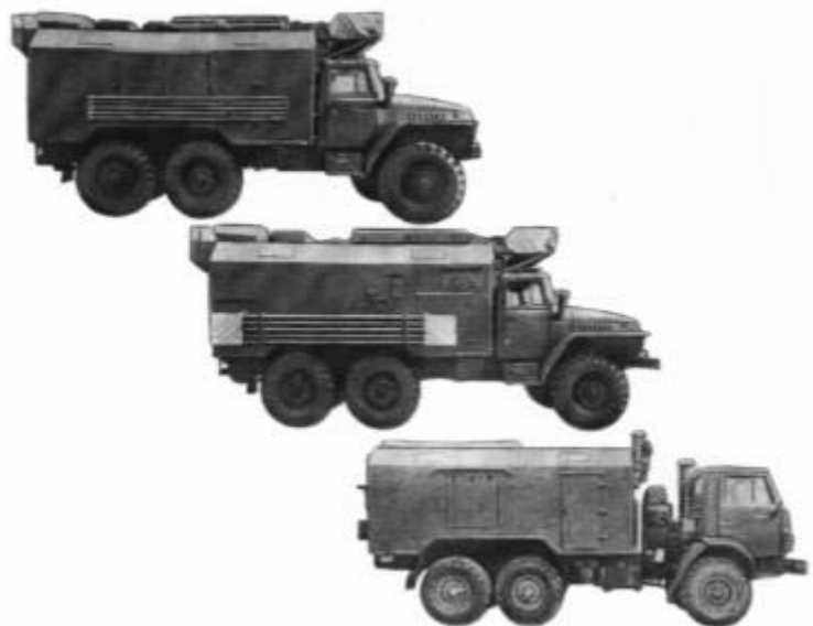
Automated Adaptive Mobile H.F. Radio Station
