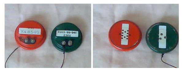
These inserts can be positively identified by measuring the DC resistance which will be 42 ohms at around 20 degrees C.
