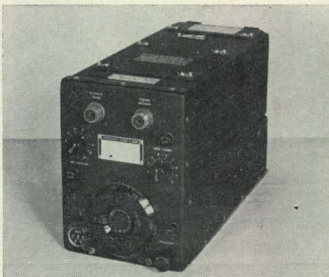
This T-90/ARC-5 was the last of the WW II command transmitter designs, covering 125-156 mc.
