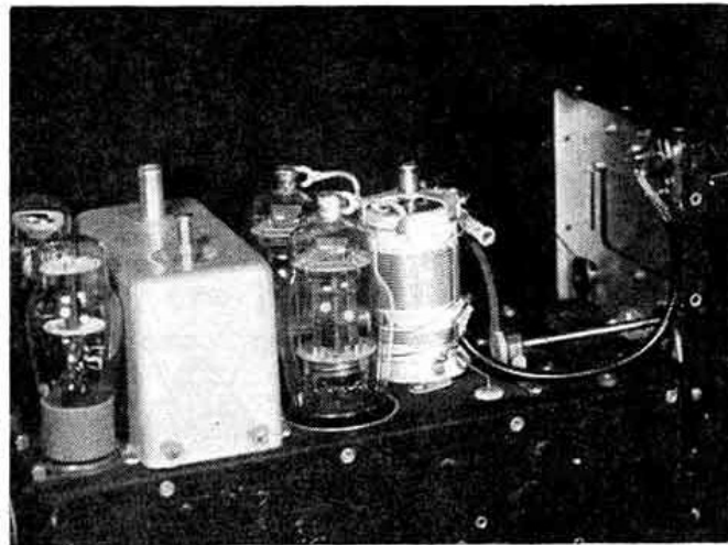
Above-chassis view of a modified unit, showing the co-axial cable from the coupling link to the output socket on the front panel. Note that the vertical wire on the side of the p.a. tank coil is at high r.f. potential, and great care should be taken that the co-axial cable outer braiding does not touch it.
