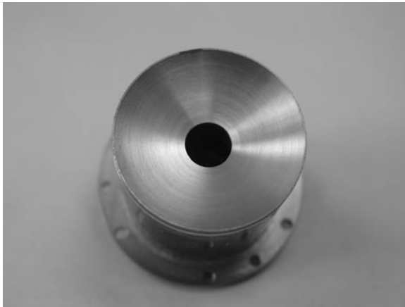
Figure 22: Tungsten Matrix (Dispenser) Cathode from a K2 series Inductive Output Tube.
