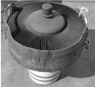
Figure 75 Example of a badly overheated tetrode. The anode fins are badly oxidized and distorted because of inadequate air flow.
