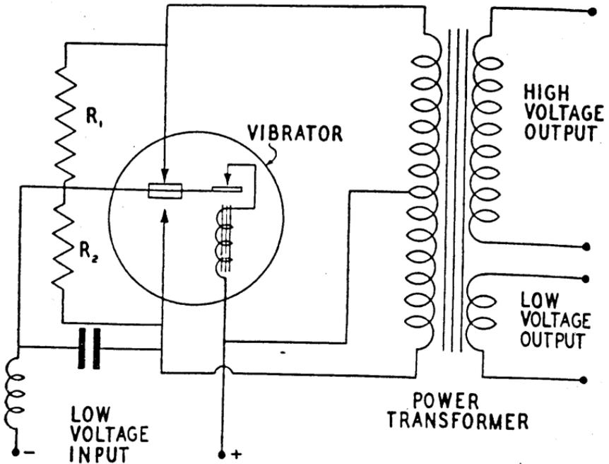
FIGURE 18. Nonsynchronous vibrator circuit.
