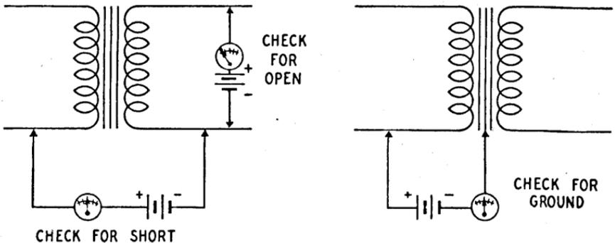
FIGURE 9. Testing transformer with continuity indicator.
