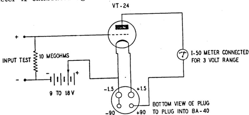
FIGURE 2. Improved vacuum tube voltmeter.
