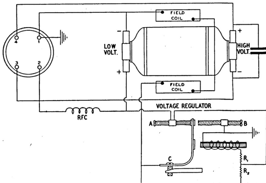
FIGURE 16. Generator circuit.
