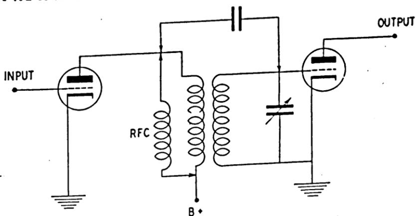
FIGURE 45. Expedient repair of transformer primary.
