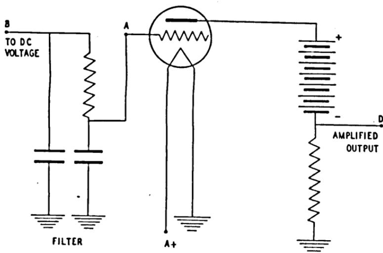
FIGURE 34. DC amplifier stage.
