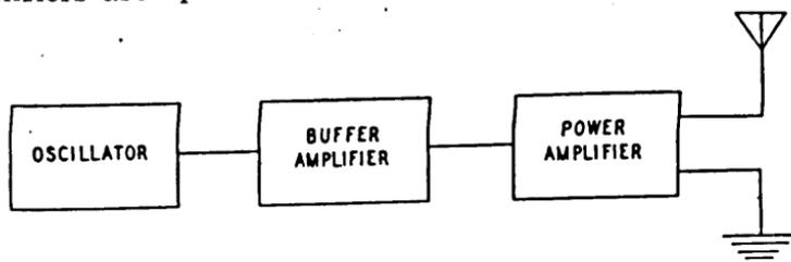
FIGURE 35. CW transmitter block diagram.
