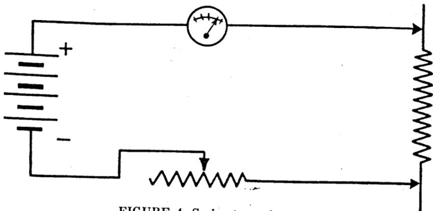
FIGURE 4. Series type ohmmeter.
