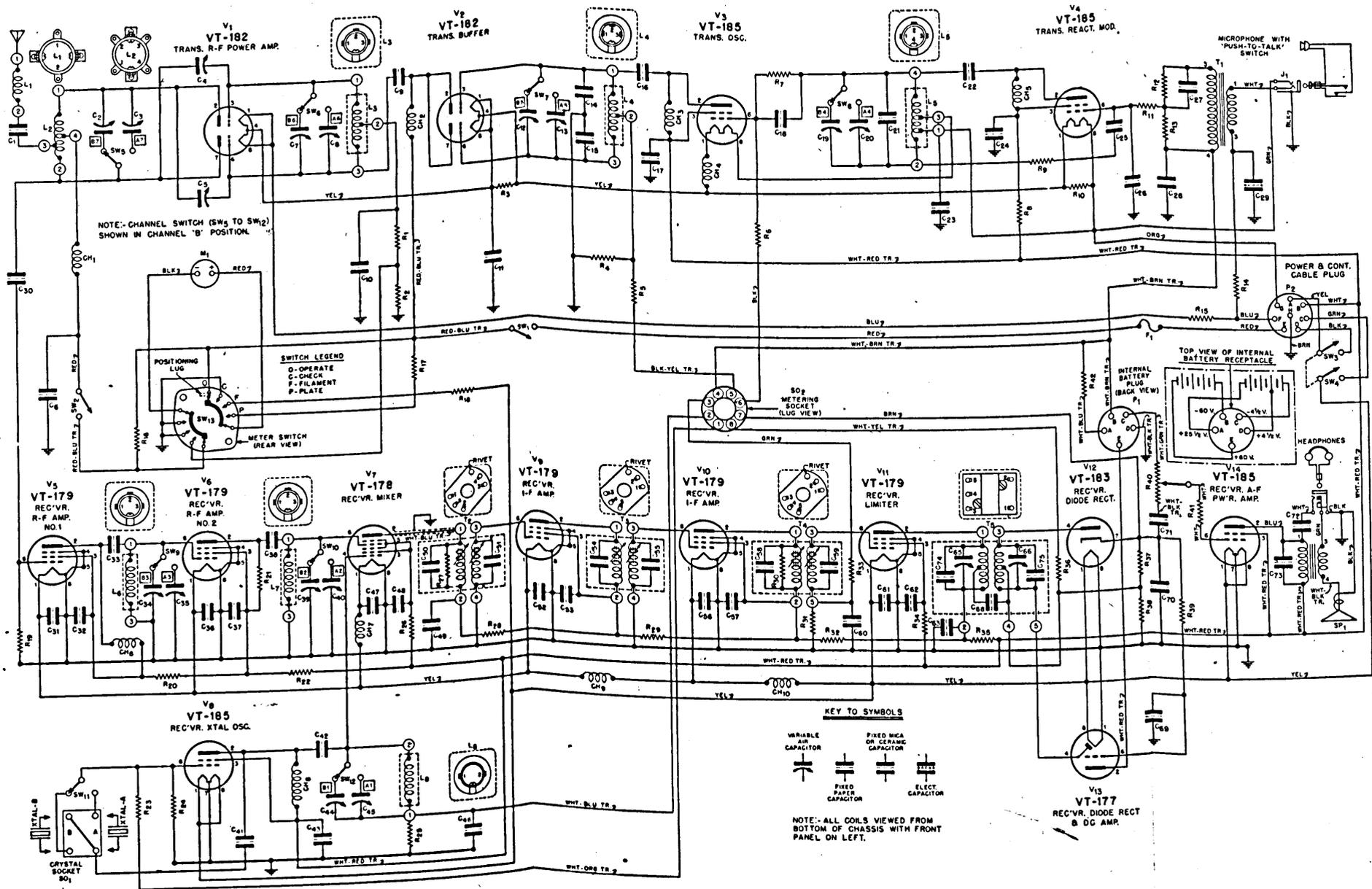
FIGURE 51. BC-659-A Transmitter and Receiver - Schematic Diagram.
