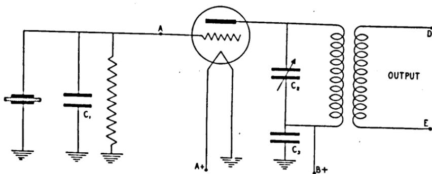
FIGURE 36. Crystal oscillator stage.
