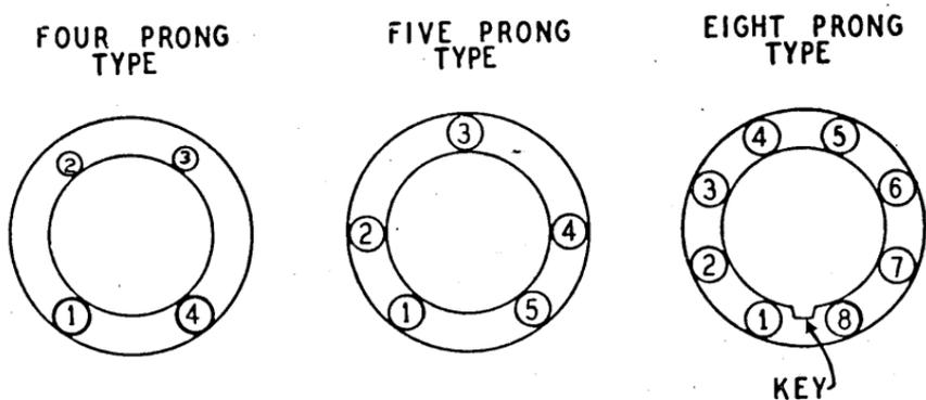
FIGURE 10. Tube base numbering system (bottom view).
