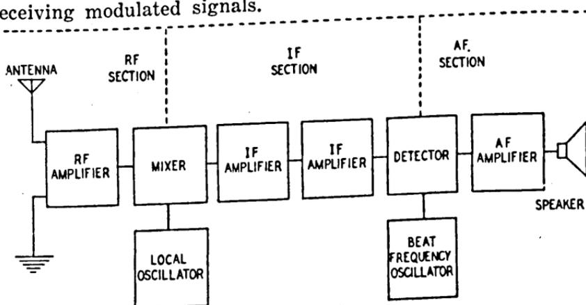
FIGURE 24. Superheterodyne AM receiver block diagram.
