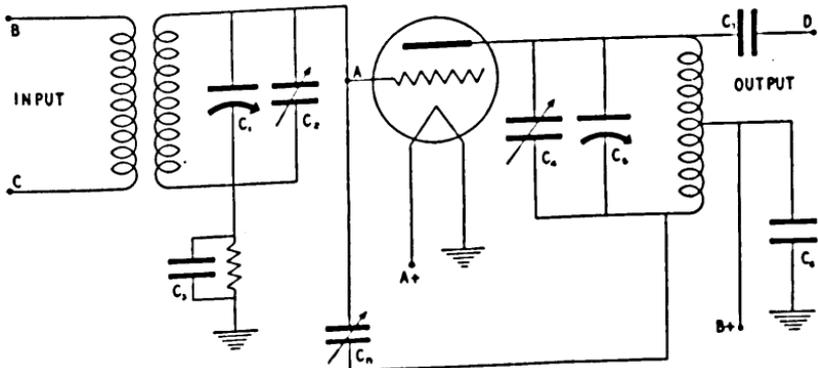
FIGURE 37. Buffer amplifier stage with plate neutralization.
