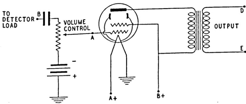
FIGURE 33. AF amplifier stage.
