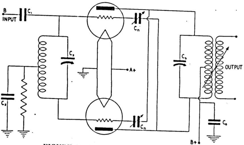
FIGURE 39. Push-pull power amplifier stage.
