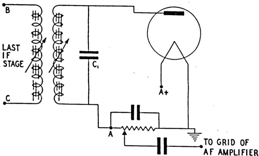
FIGURE 31. Diode detector stage.
