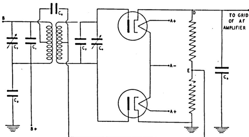
FIGURE 32. Double diode, differential discriminator stage.
