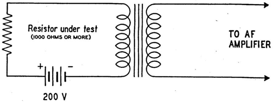
FIGURE 7. Circuit for testing noisy resistors.
