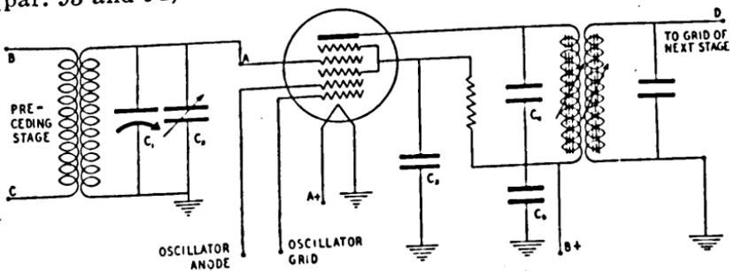
FIGURE 28. Pentagrid converter stage.
