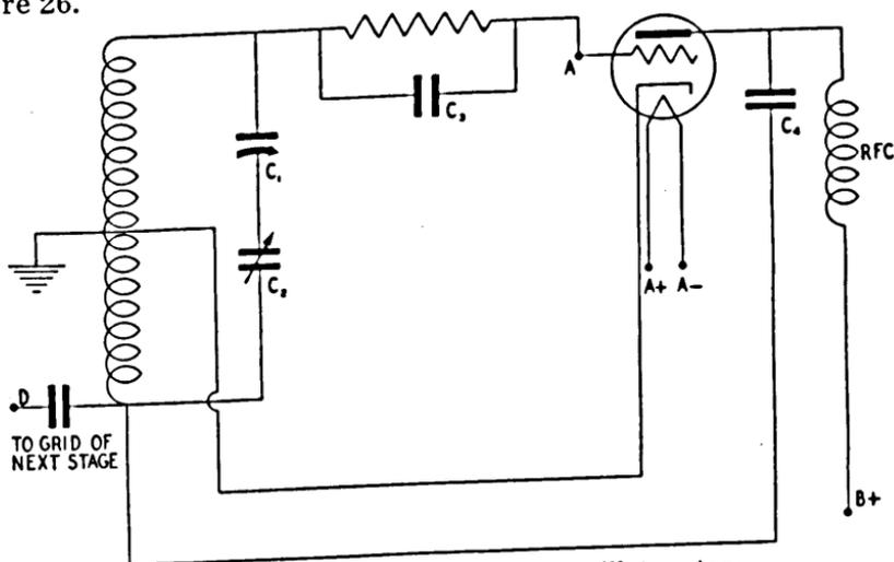
FIGURE 26. Shunt fed, Hartley oscillator stage.
