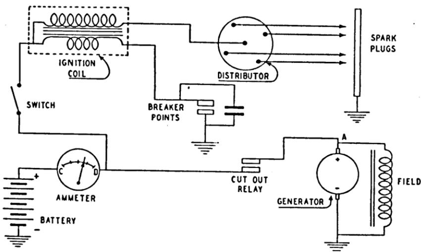
FIGURE 48. Simplified vehicle electrical system.
