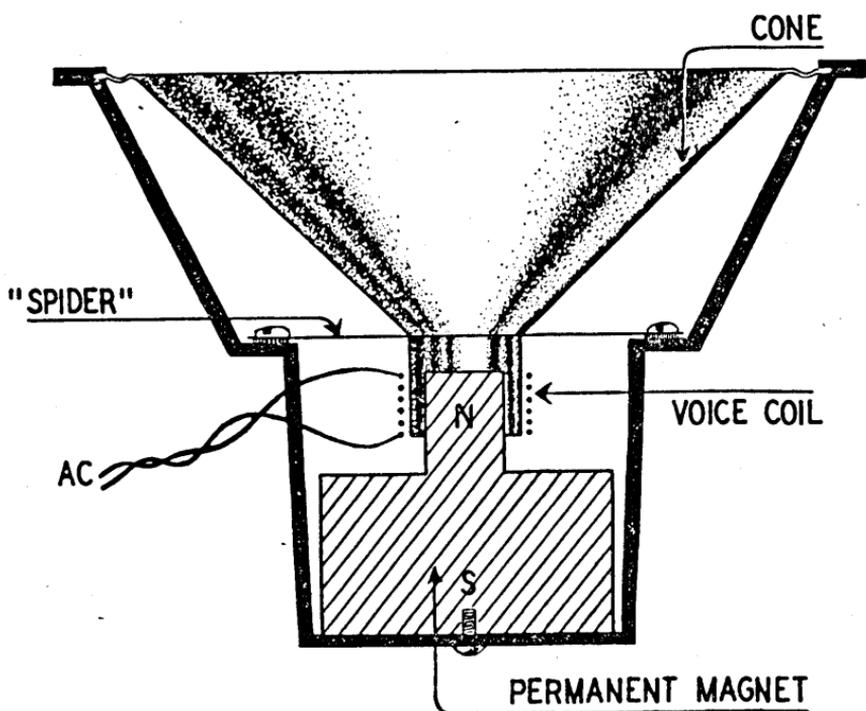
FIGURE 12. Permanent magnet, dynamic speaker.
