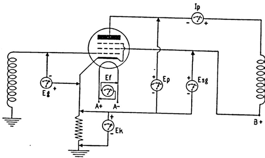
FIGURE 42. Meter connections for checking pentode stage.
