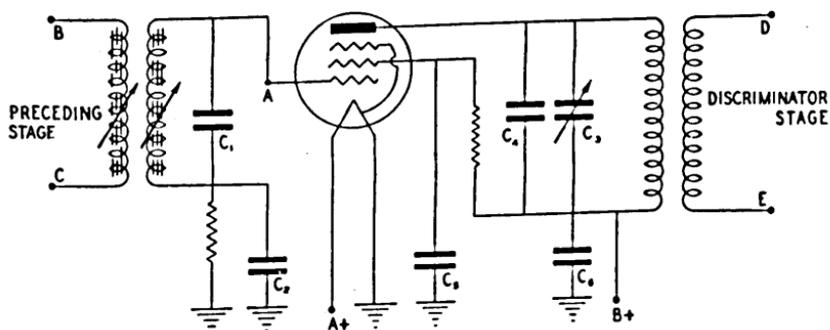
FIGURE 30. Limiter stage.
