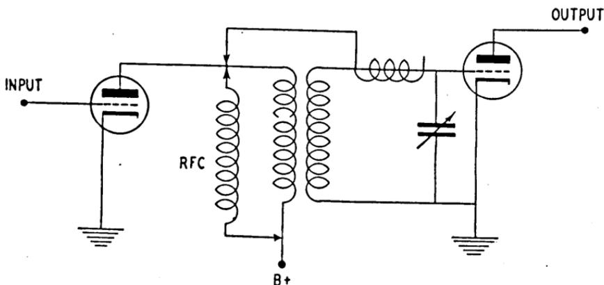
FIGURE 46. Improved coupling condenser.
