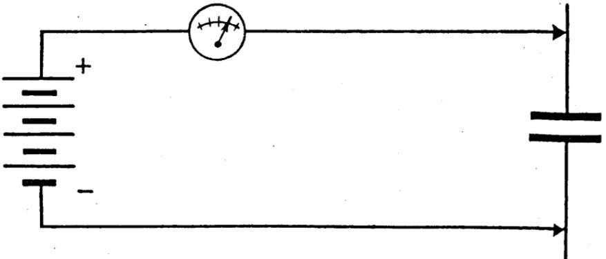
FIGURE 8. Condenser working voltage test.
