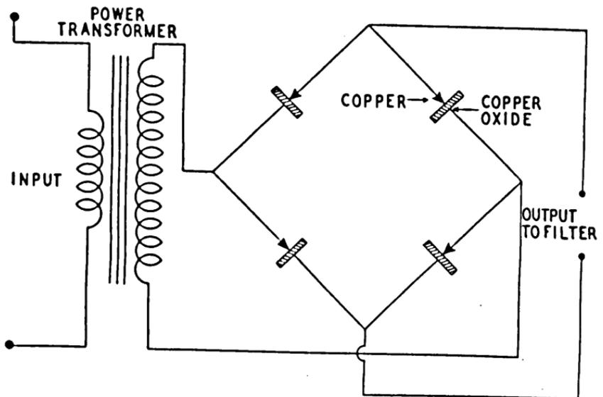
FIGURE 21. Full-wave bridge rectifier.
