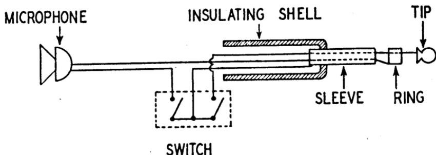
FIGURE 13. T-17 Microphone circuit.
