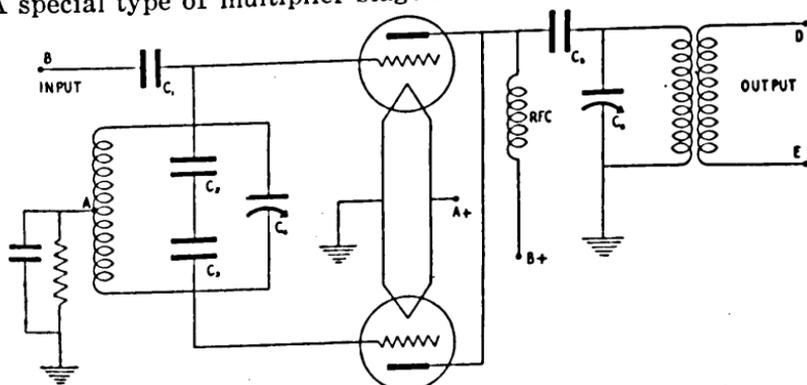
FIGURE 38. Push-push frequency multiplier circuit.
