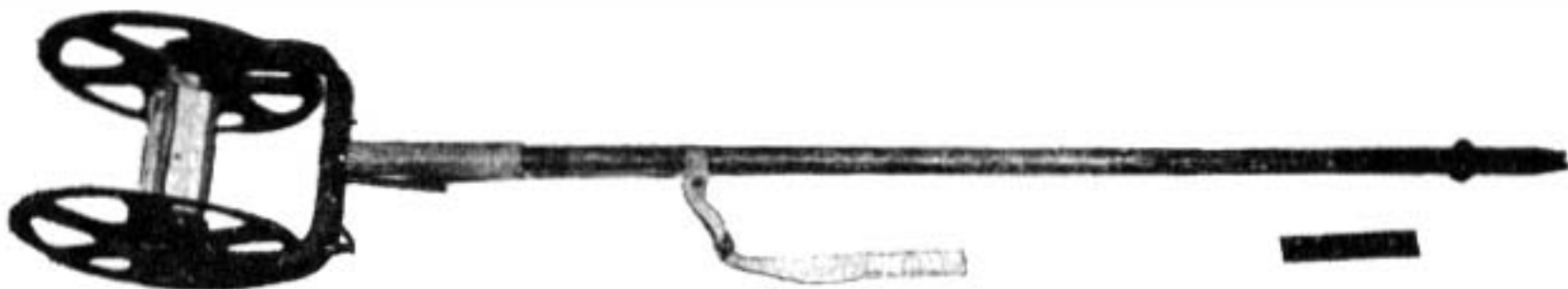
Figure 371. Hand wire reel unit with broomstick handle.
