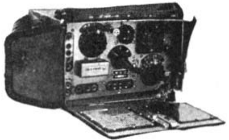
Figure 343. Model 94 Type 5. Transmitter-receiver Model 32. Transmitter. Operates C.W. or phone. Used with receiver shown below.
