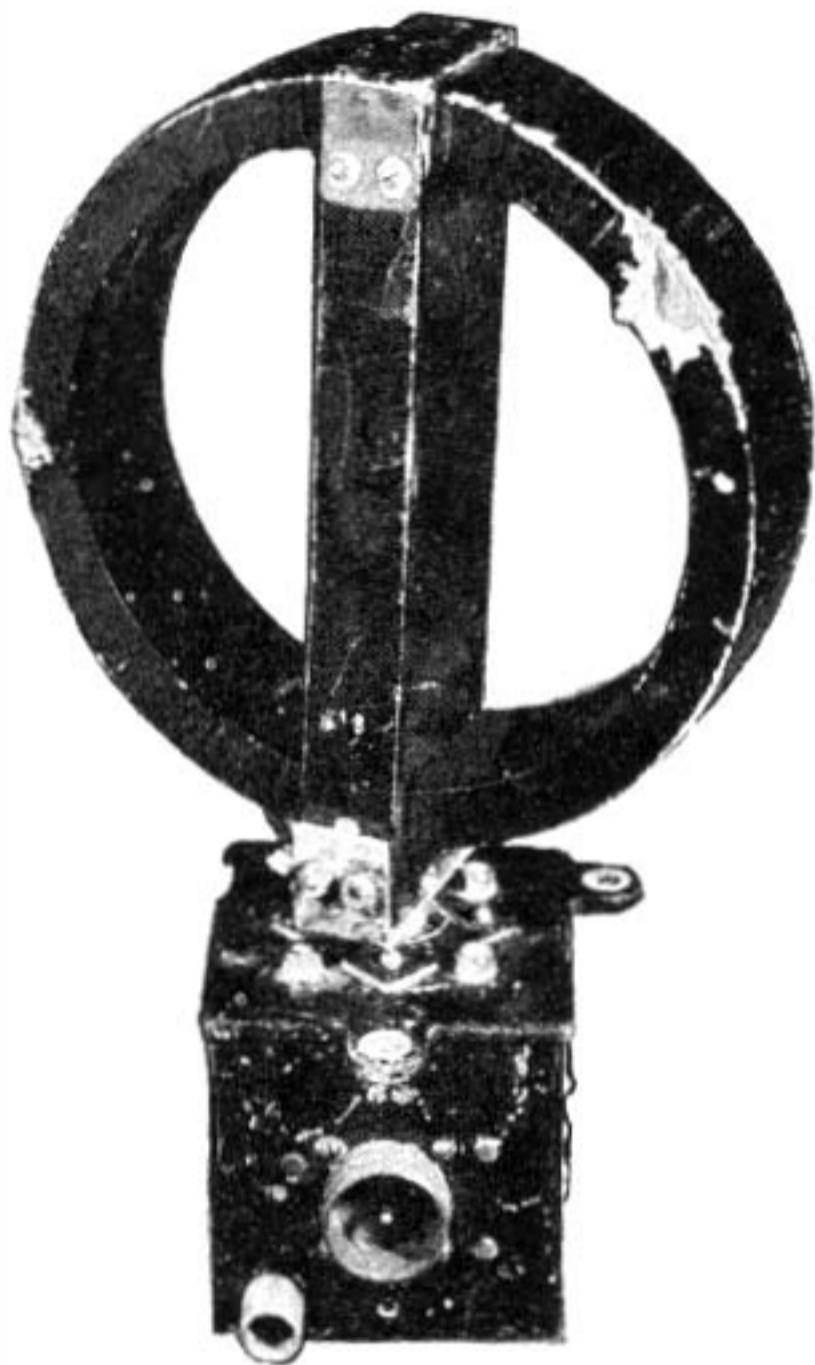
Figure 356. Radio Hanning and D/F loop antenna used with some types of Japanese airborne equipment.
