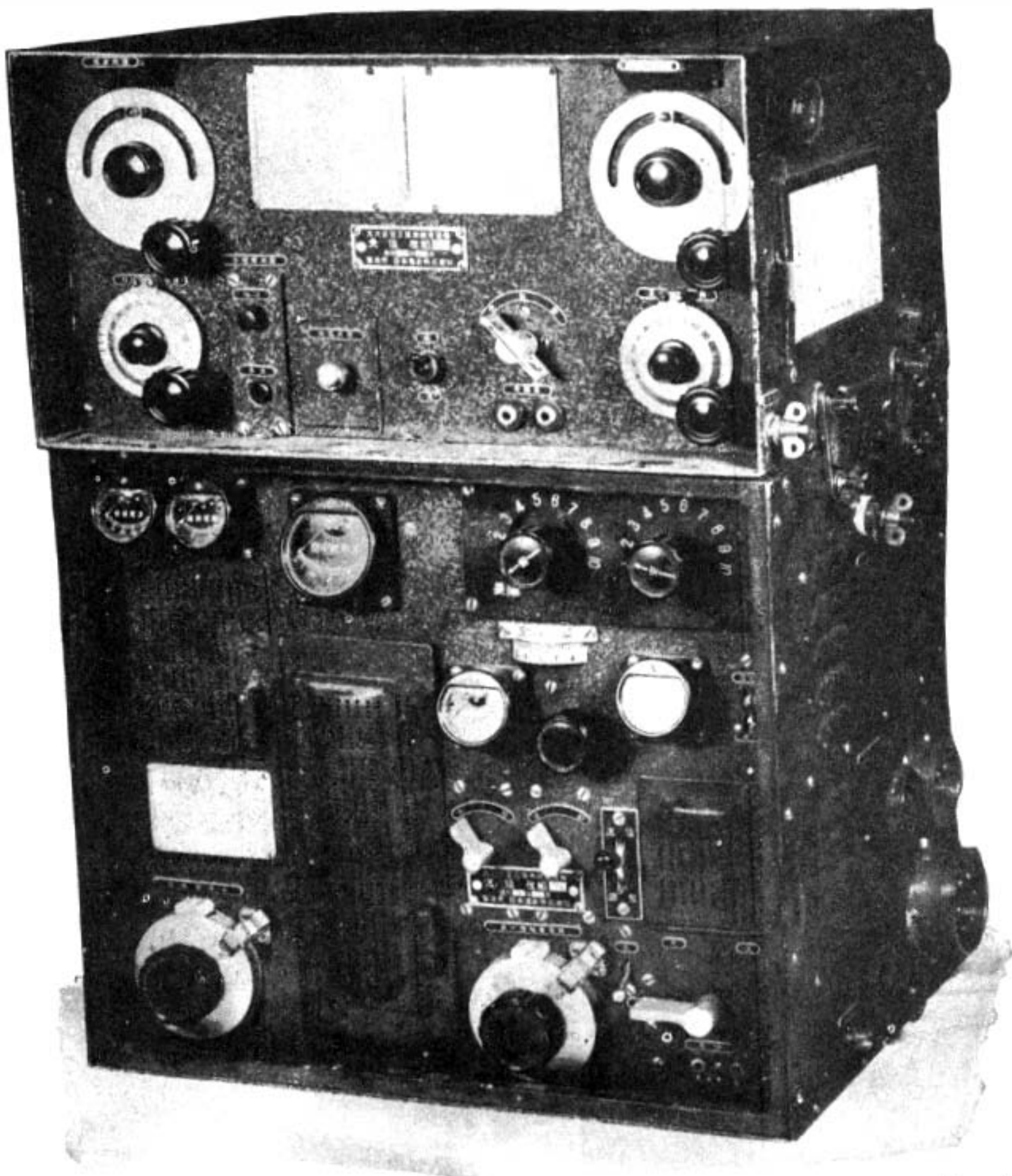
Figure 355. Model 96 (1936) Type 3. Transmitter-receiver. From Type 1 medium bomber (B-25). Top of unit: receiver. Bottom of unit: transmitter.
