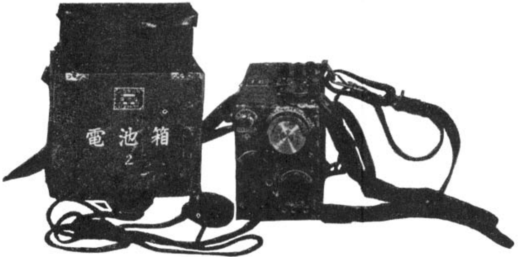
Figure 347. "Walkie Talkie" Type 66. Transceiver. Model A. 2500-4500 KC. Power supply—batteries.
