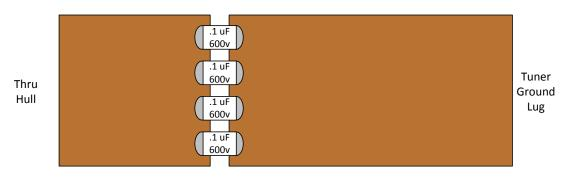
The following information is from Cruiser's Forums User *transmitterdan*. Information on why one would use coupling capacitors or DC block capacitors is readily available on the web for your education. The primary purpose is to prevent galvanic corrosion by mixing AC currents with DC currents.
